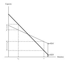
Two load duration curves and the corresponding technological mixes With a more variable load there are more peakers and less baseload units.
